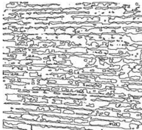
Figure 4. Image of the binary surface, corresponding to the image shown in Figure 3, by which the fractal dimension was determined
